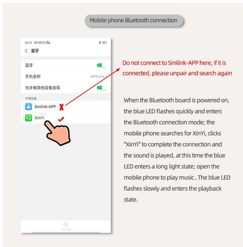
Make sure that Bluetooth enters Bluetooth connection mode-blue LED flash, AUX do not insert, can not enter Bluetooth connection state after insertion
