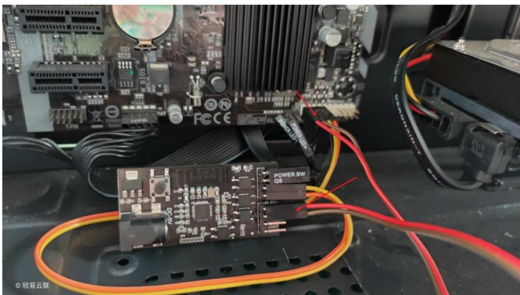
6. Pull out from the motherboard with POWER LED + DuPont to PLED1, with POWER LED-DuPont to PLED2(in sequence with step 5);
