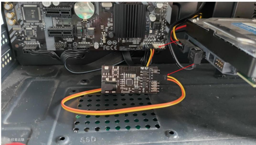
3. Connect the connector for the POWER SW removed from the motherboard to the product P-KEY position; as shown in the figure below
