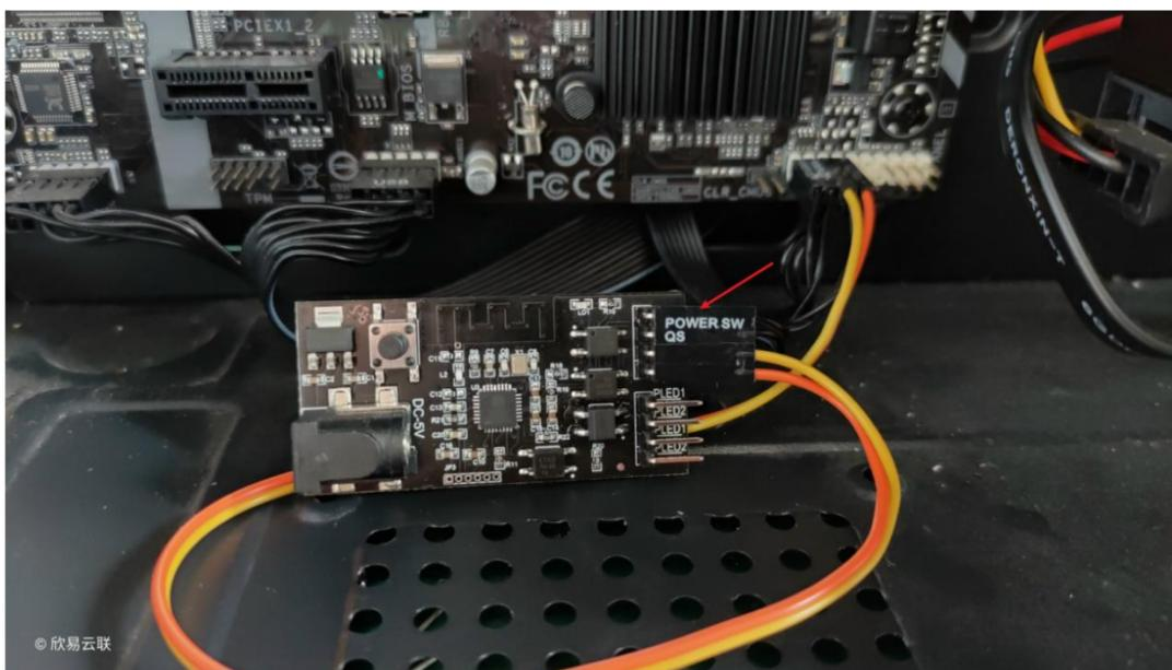
4. Locate the connector with POWER LED + and POWER LED- on the motherboard, pull it out and plug the presented bus DuPont line, remember the positive and negative order (red- -LED + gray- -LED-) (note: its words, not HDDLED, and remember the extraction position)
