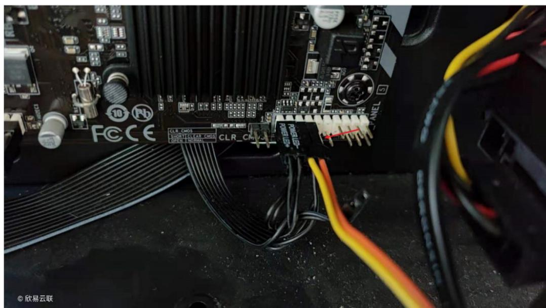
2.Connect the other end of the attached DuPont line to P-SW on the product; as shown in the figure below
