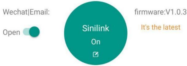
1. Open the APP into the device operation interface, the top left corner is the switch of the mail notification function; if the email notification is turned on, when the computer status sends the change will send the latest status and operation type of the computer in real time through the mailbox used to register the APP;
